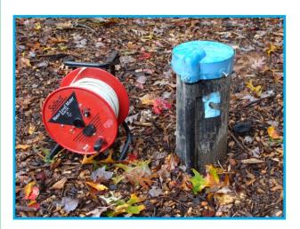
New drilled well at the Annex reported to be 300 feet deep. The water level in the well is 58.78 ft below the top of the casing at an elevation of 16.82 ft msl, some 50 feet below the surface of Wash Pond. Thus, this well draws its water from a deep, confined, aquifer isolated from the glacial kettle ponds.
